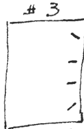
thru board twice top & bottom at angle
